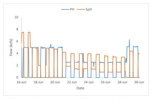
Figure 54. Hourly Flows PWR vs. Spill (Lookout Dam Tailrace)
