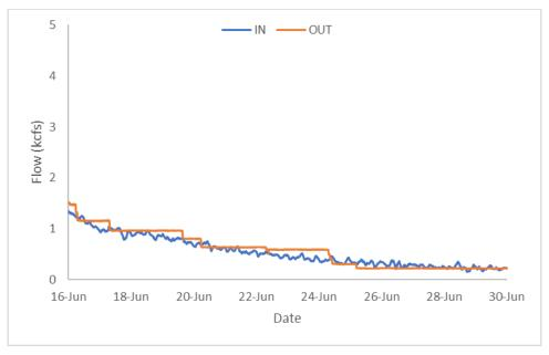
Figure 42. Hourly Flows IN vs. OUT (Fall Creek Tailrace)
