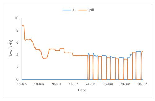
Figure 48. Hourly Flows PWR vs. Spill (Dexter Dam)
